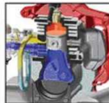
COMBUSTION Crankcase is filled with air while injection tube draws fuel
